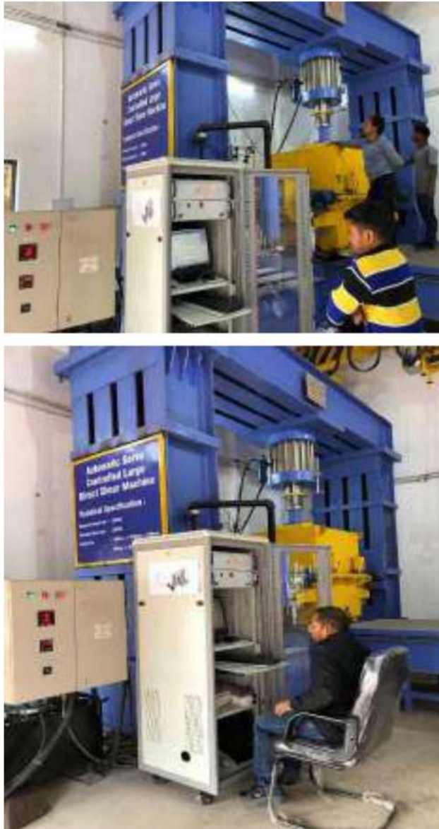
Figure 5.2 Pictures showing sample testing on Large Direct Shear Machine, CMPDI
