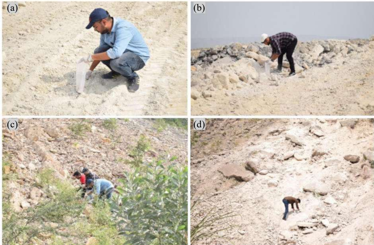
Figure 5: Collection of samples from the East Overburden Dump for Leachate and Runoff Analysis. (a-b) Collection of Overburden material from the top of the dump (c) Collection of Overburden material from the middle of the dump (d) Collection of Overburden material from the toe of the dump.
