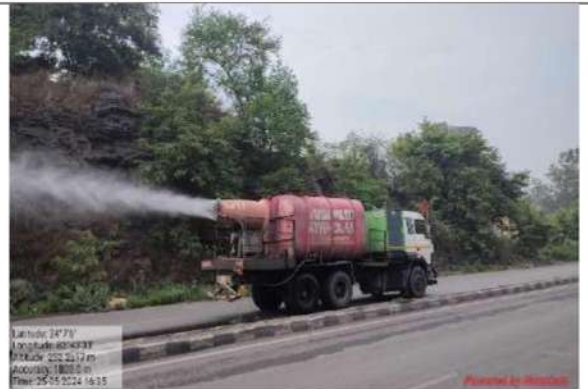
Pic 18 Deployment of truck mounted fog cannon on public road
